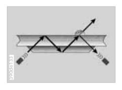
When the system is set to the "Intermittent" wiper speed, the wipers react immediately – if water is splashed onto the windshield by vehicles traveling ahead of you, for example. As a result, the rain sensor provides a contribution to driving safety and comfort.
