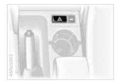
The push button flashes rhythmically when the hazard flashers are on.
