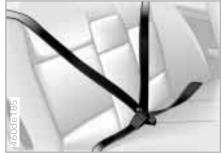
If you are transporting very heavy loads when the rear seat is not occupied, secure the outer safety belts in the opposite buckles (refer to the illustration).
