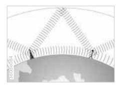
AM radio provides reception across a considerable distance because the broadcast signals not only travel along the ground as surface waves, but they are also reflected from the ionosphere as atmospheric waves.
