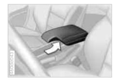
Open the storage compartment in the front center armrest\*: Press the button (arrow) and lift upward.
