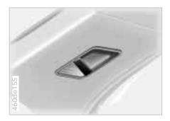
The reading lamps are located in the front\* near the interior lamp and in the rear\* (illustration). They can be switched on and off with the switch adjacent to each lamp.
