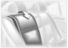
The rear backrest section will move forward slightly when it is unlocked. Reach into the gap and pull the backrest down.
