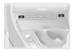
The seat cushion and backrest can be heated with the ignition key in position 2.
