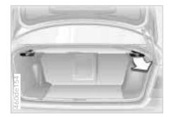
The rear backrest is divided into two sections (one-third and two-thirds of the width of the seat). For carrying longer objects, you can fold down either section of the backrest separately.
