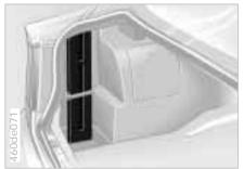
The hazard warning triangle is stored in a recess on the left-hand side of the luggage compartment where it is quickly available.
