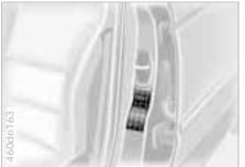
The inflation pressures are indicated on a sticker attached to the door pillar behind the driver's door (visible with door open).
