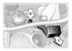
gine compartment. The cover of the positive terminal connector is marked with a "+" sign. Refer to the illustration. Remove by pulling the tab (arrow 1).
