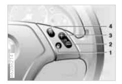
You can store and automatically maintain any desired vehicle speed above approx. 20 mph (30 km/h).
