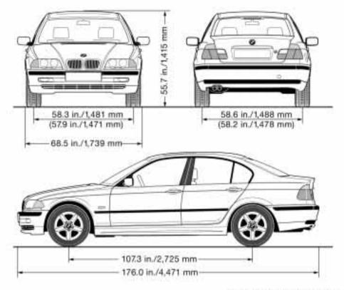
Dimensions in () apply to 328i. Minimum turning circle dia. 34.4 feet (10.5 m).
