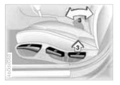
3 Backrest angle Pull the lever and apply weight to or remove weight from the backrest as required.
