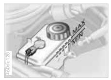
If the brake warning lamp comes on and the parking brake has been released:
