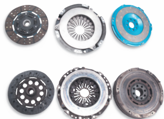
Bottom row: old, worn SAC and dual-mass flywheel. Top row: new UUC performance clutch and lightweight flywheel.
