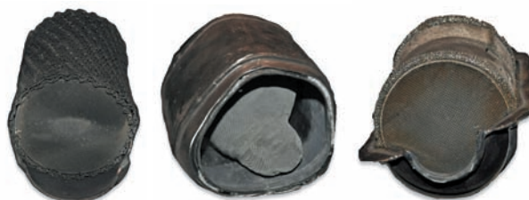
Above left: a catalytic converter that is covered in carbon caused by too rich a fuel mixture. Above middle: a catalytic converter that has overheated/ melted due to too lean a fuel mixture. Above right: typical appearance of a properly maintained catalytic converter.
