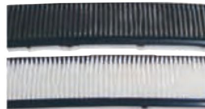
The top filter was pulled out of a 1999 323i after 30,000 miles; the bottom filter is new. Not only is cabin air healthier with a new filter, it smells better.
