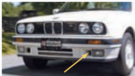
Driver's side, under bumper, in valance panel or brake duct: 3 series thru 91, 5 series thru 88, 6 series thru 89, 7 series thru 87.
