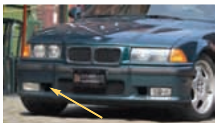
Passenger's side brake duct: 3 series 92 thru 98.
