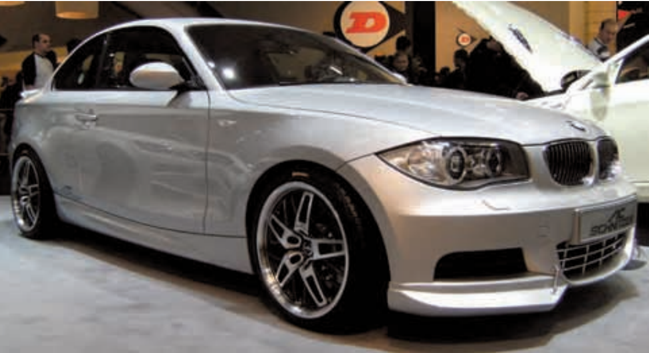
AC Schnitzer's ACS1 3.5i, based on the stock 135i with M-Technic styling, features a front grill, front lip spoilers with stabilizers and 18" Type VI wheels.
