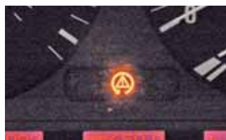
Top: the DSC button in a 2001 540i. Bottom: traction control indicator light.
