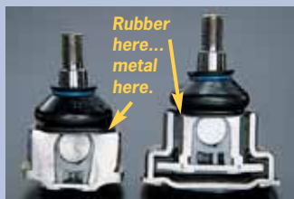
Meyle's all-metal ball joint is on left; BMW's OE ball joint is on the right.
