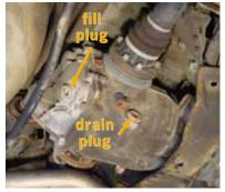
has any leaks, the fluid level should be checked Rear differential on a 3 series 99 thru 05.
