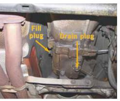
Manual transmission on a 1999 323i. Fill plug and drain plug are indicated with arrows.
